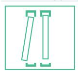
You will receive two channels - one being slightly bigger than the other. Screw the middle of the bigger channel to the top of your recess and the smaller one to the bottom.
